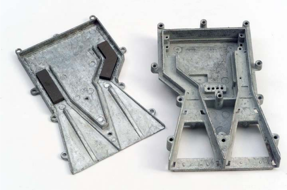
Figure 4. A thin, flexible broadband absorber like ECCOSORB® MCS exhibits a high permittivity and permeability, as well as magnetic loss tangent, making it ideal for cavity resonance dampening in military applications like radar systems.
